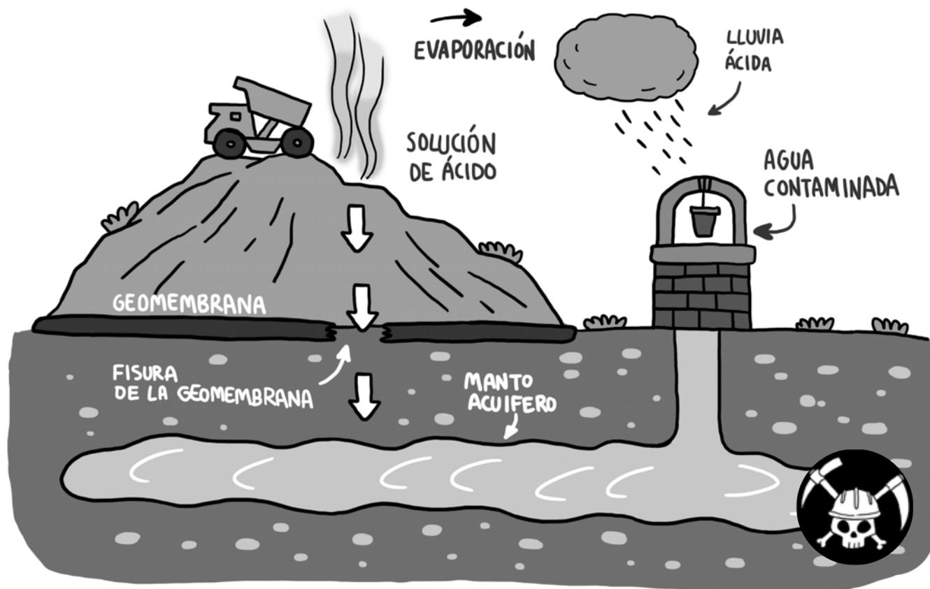
"DRENAJE ÁCIDO EN UNA MINA A CIELO ABIERTO"<sup>11</sup>
